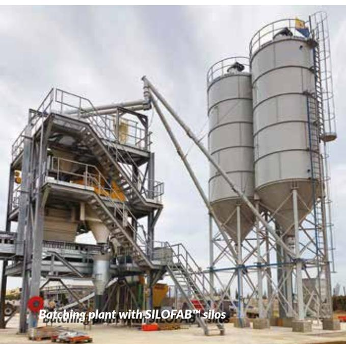
Batching plant with SILOFAB™ silos
