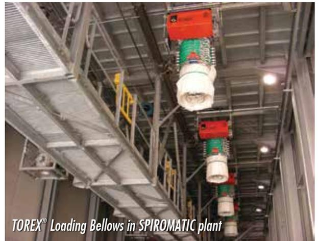
TOREX<sup>®</sup> Loading Bellows in SPIROMATIC plant
