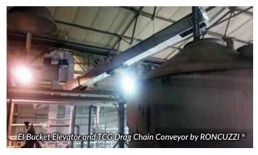
Earlier this year, WAM Romania Trading received an enquiry from Kronospan in Sebeş, a manufacturer of wood boards, worktops, panels, edgings, foils, high pressure laminate (HPL), and lacquered high-density fireboard (LHDF). For the production of wood glue, urea granules are an important ingredient of the recipe. To convey the granules from the storage tank to the reactor vessel mechani-
